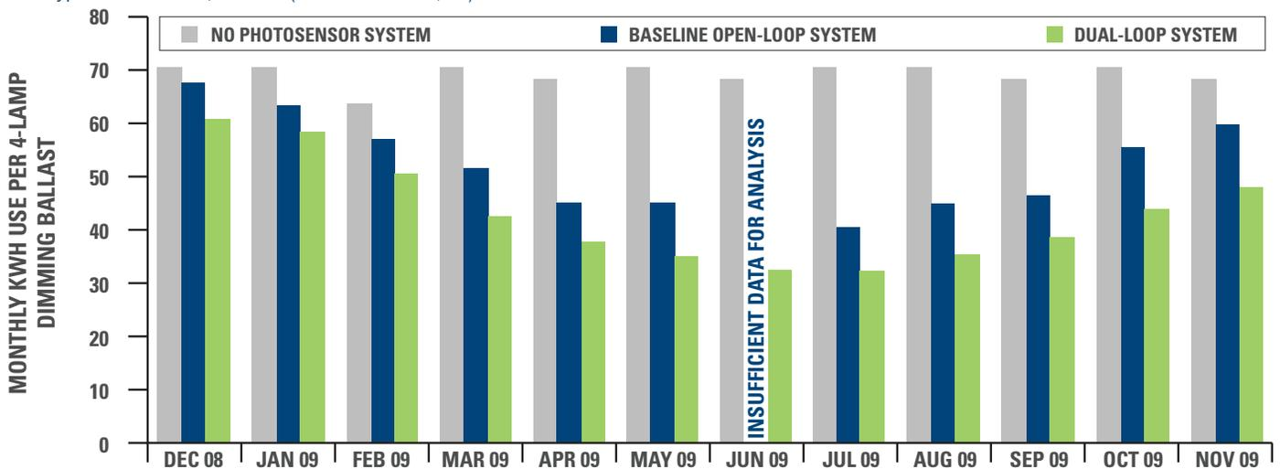
This chart compares energy savings between the dual-loop and the open-loop systems. The open-loop system saved 24.4% over a store without a photosensor system while the dual-loop system saved 36.6% over a store without a photosensor system, a 50% improvement in the energy savings achieved by the baseline technology.
