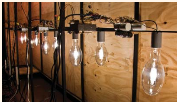
FIGURE 1: PHILIPS ENERGY ADVANTAGE CDM LAMP WITH ALLSTART™ TECHNOLOGY LAMP TESTING AT CLTC
