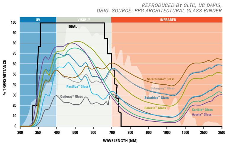
**FIGURE 44** Spectral transmittance of tinted glass and various spectrally selective glazings.
