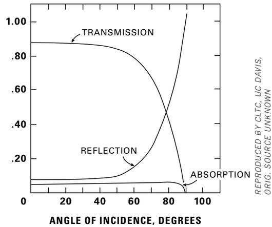
**FIGURE 38** Single-pane clear glass optical and solar properties as functions of incident angle on the glass surface.
