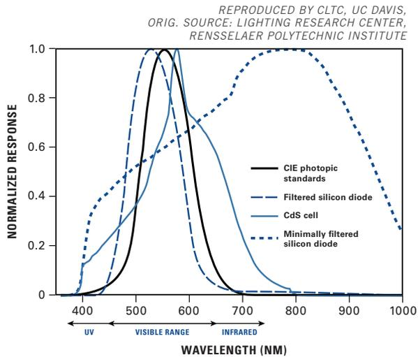
**FIGURE 69** Spectral sensitivity of different light sensing technologies, along with the human Photopic sensitivity standard. Photosensors that deviate from the Photopic sensitivity, such as those that use a minimally filtered silicon diode, can be unreliable, as their signal is affected by non-visible radiation.
