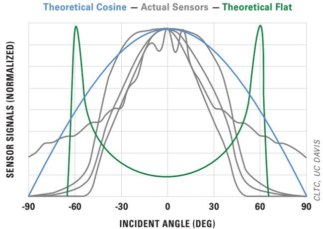
**FIGURE 70** Directional sensitivity of various commercially available photosensors, along with a cosine response, where the sensitivity drops by the cosine of the incident angle, and a “flat” response, which is a computed sensitivity aimed at producing the same signal from all incoming directions within a confined field of view (FOV).
