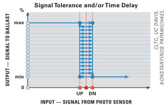
**FIGURE 76** Schematic diagram showing the operation of typical constant set point algorithms, which is realized either by setting a time-delay before taking action after a deviation of the photosensor signal from the set point, or by setting a range that defines the maximum allowable deviation from the set point.
