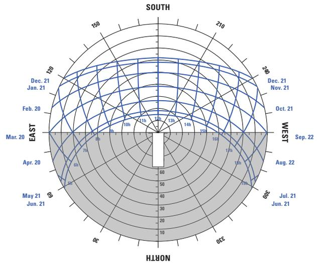
**FIGURE 24** South-facing apertures in California are exposed to direct sun throughout the day during the fall-winter-spring periods. The winter sun directions are from very low solar altitude angles and can produce significant flare. The sun exposure during the summer occurs only during the middle of the day and from very high solar altitude angles, resulting in high incident angles on vertical apertures.
