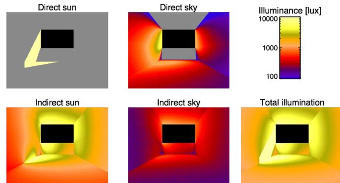
**FIGURE 60** Daylight simulation results showing the contribution of the direct and reflected sun and sky components on the brightness of interior surfaces.
