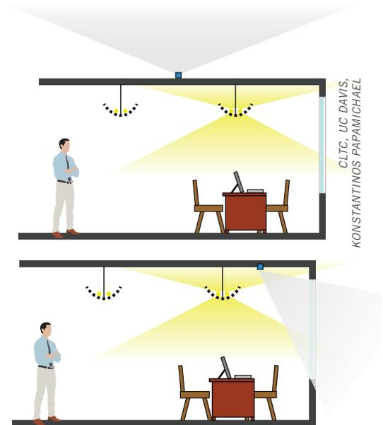
**FIGURE 71** Schematic drawings showing placement and field of view of photosensors for open-loop photo sensing.
