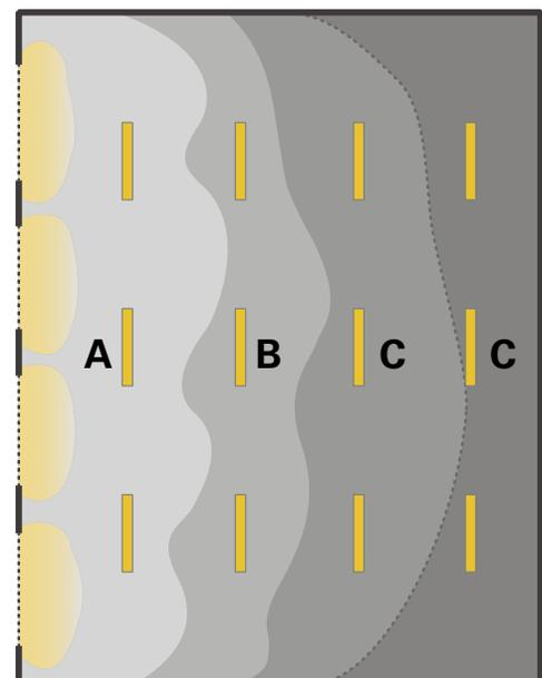
**FIGURE 64** Schematic drawing showing layout of electric lighting luminaires parallel to the window wall and organized in three groups that are controlled individually to effectively account for available daylight levels, which drop significantly as the distance from the window wall is increasing.
