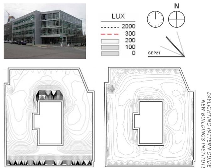
**FIGURE 20** Rectangular foot-print building with atrium, resulting in 100% and 90% of floor space being adequately illuminated by daylight under sunny and overcast conditions, respectively, on September 21 at noon.
