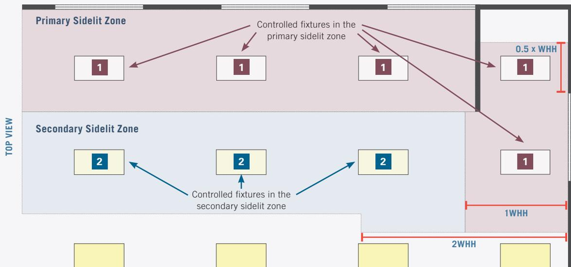
**FIGURE 68** Example electric lighting and daylighting design used to show how to calculate a primary and secondary sidelit zone with a permanent obstruction that is 6 feet.
