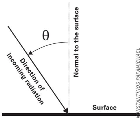
**FIGURE 34** The incident angle of radiation on a surface is the angle of the direction of incoming radiation from the normal direction to the surface. It varies from 0 (coincident to the normal direction) to 90 degrees.
