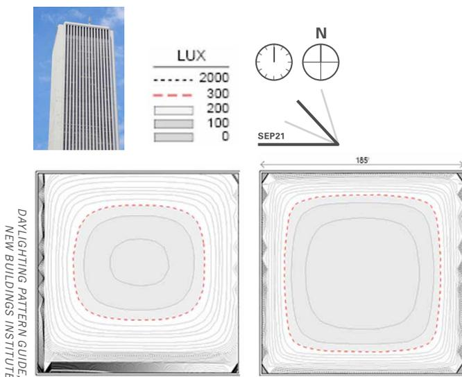
**FIGURE 19** Rectangular foot-print building with large core area, resulting in 55% and 25% of floor space being adequately illuminated by daylight under sunny and overcast conditions, respectively, on September 21 at noon.
