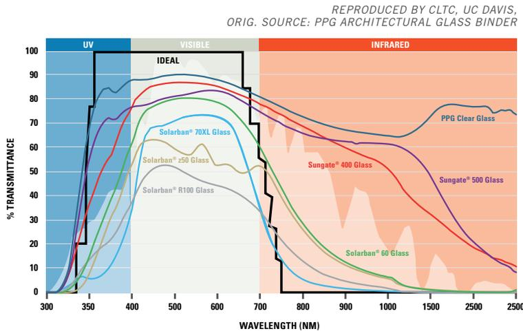
**FIGURE 43** Spectral transmittance of clear glass and various spectrally selective glazings.
