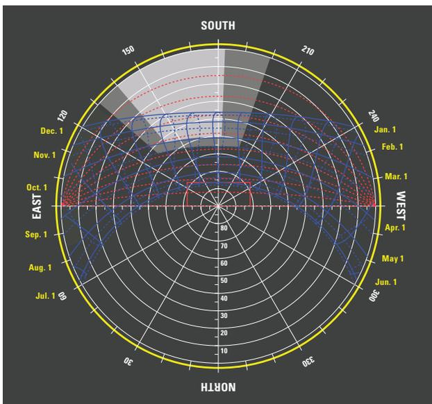
**FIGURE 15** Full and center point shadow masks for a daylight aperture.
