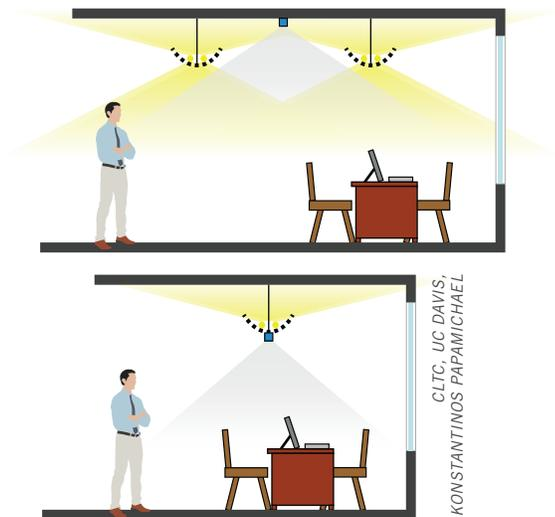
**FIGURE 72** Schematic drawings showing placement and field of view of photosensors for closed-loop photo sensing.
