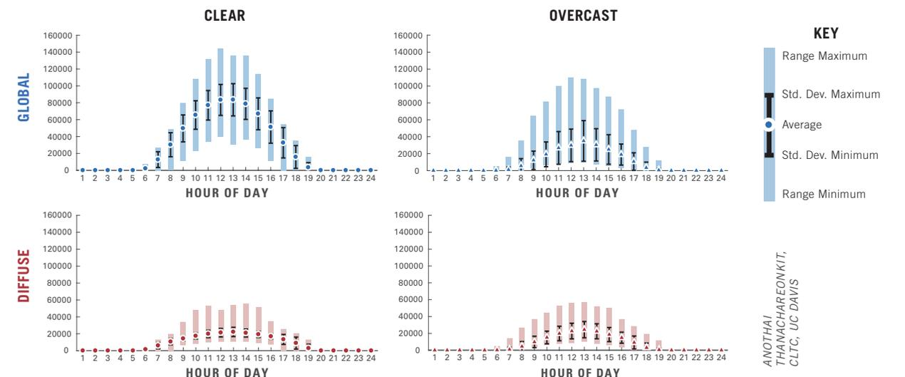
FIGURE 12 Average hourly horizontal daylight illuminance for Sacramento, California, from global (sun and sky) and diffuse (sky only) radiation under clear and overcast sky conditions. The data show average values for each hour, along with standard deviation, minima and maxima. Overcast sky conditions from global radiation result in higher illuminance values than clear sky conditions from diffuse radiation.
