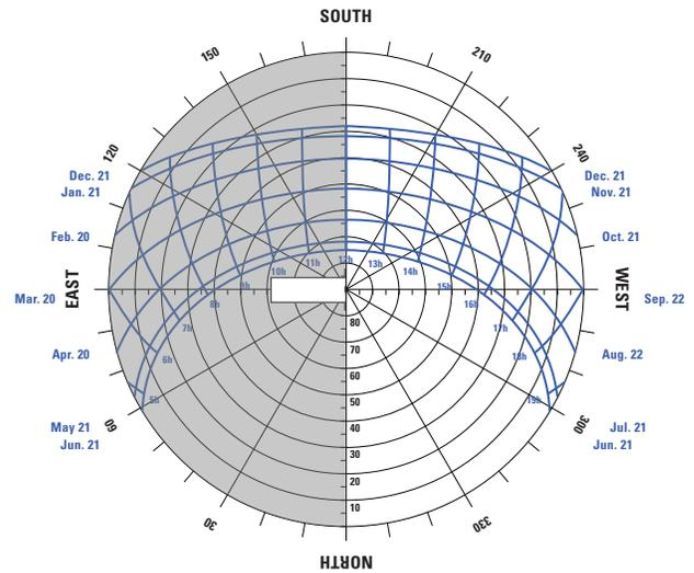
**FIGURE 25** East- and West-facing apertures in California will be exposed to direct solar radiation only during the morning and afternoon hours, respectively, throughout the year. Direct solar radiation is incident at very small incident angles for both orientations during the beginning and the end of the day, respectively.
