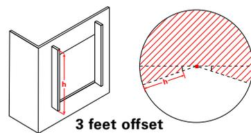
**FIGURE 54** Shadow masks of exterior overhangs and vertical fins.
