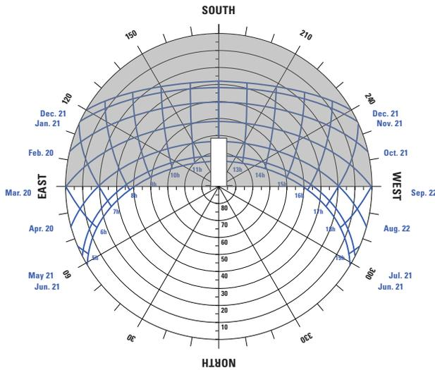
**FIGURE 23** North-facing apertures in California will be affected by direct solar radiation only during the early morning and late evening of the summer season.
