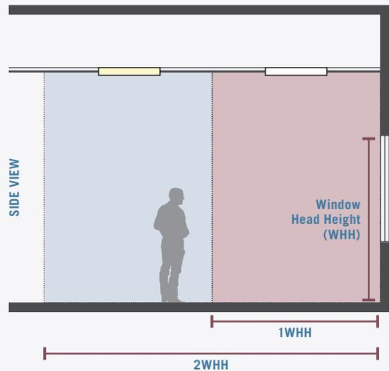
**FIGURE 67** Example electric lighting and daylighting design used to show how to calculate a primary sidelit zone.
