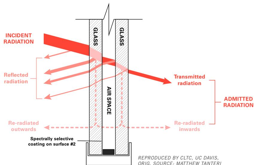
**FIGURE 36** Schematic drawing showing the transmitted, reflected and absorbed fractions of the incident solar radiation.
