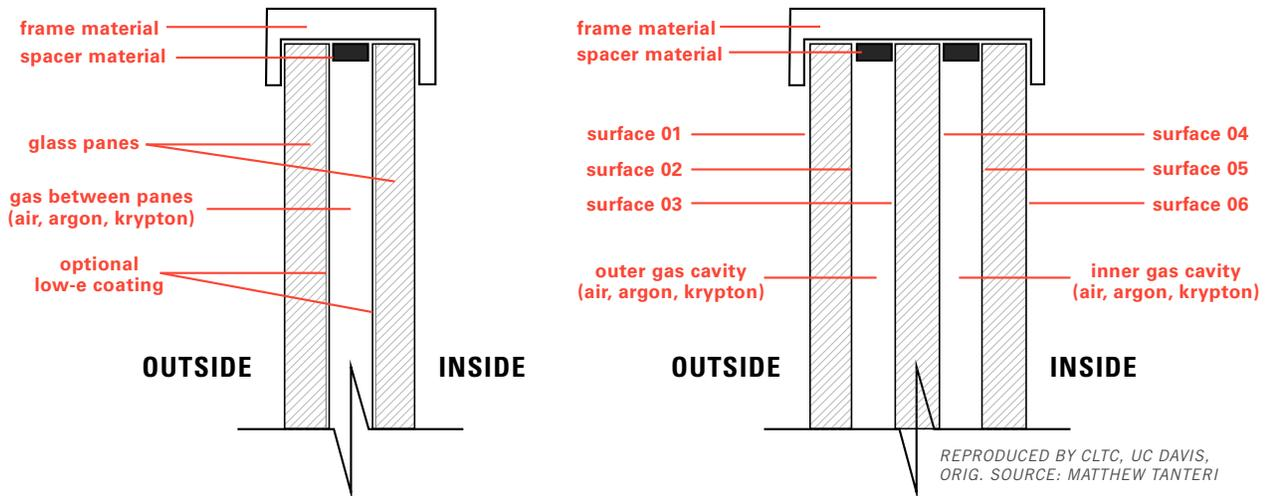
FIGURE 50 Schematic drawings of double and triple glazing systems.
