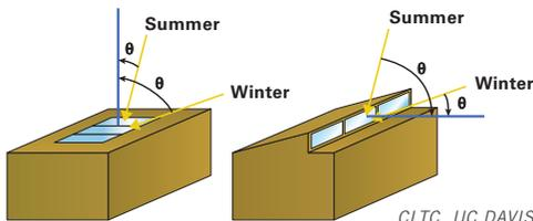
**FIGURE 39** South-facing clerestories receive more radiation per unit area during the winter than during the summer, while horizontal skylights receive more during the summer and less during the winter.
