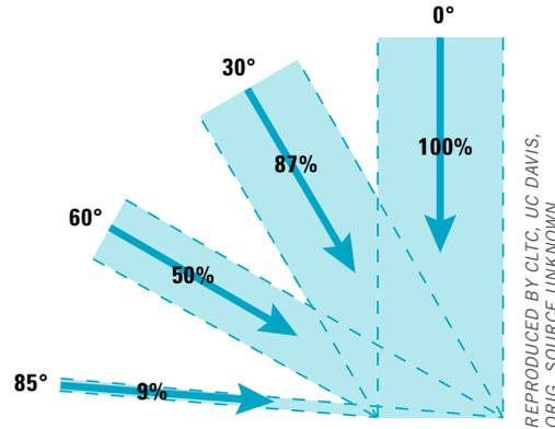
**FIGURE 37** The incident radiation per unit area decreases by the cosine of the incident angle.
