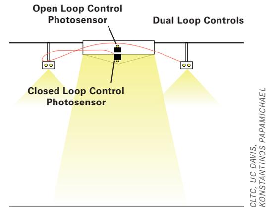
**FIGURE 80** Schematic drawing showing dual-loop sensing approach in skylight applications.
