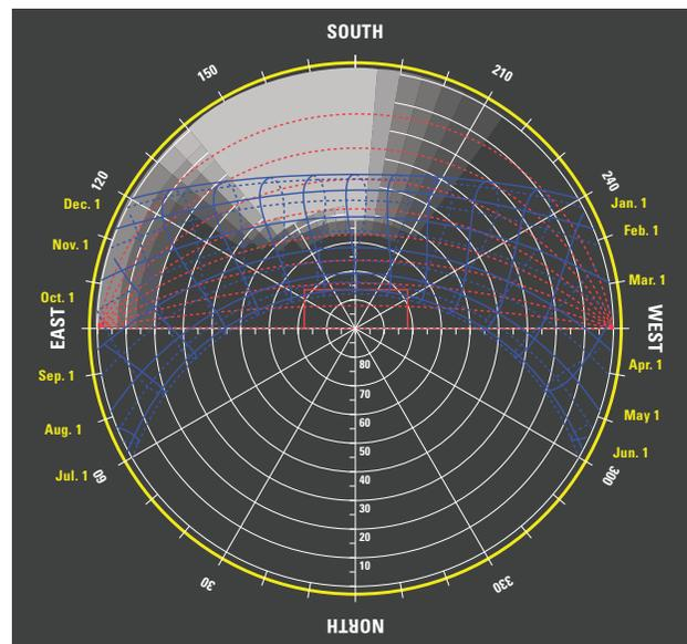
**FIGURE 16** Percent shadow mask showing the percent of the daylight aperture that is being blocked.
