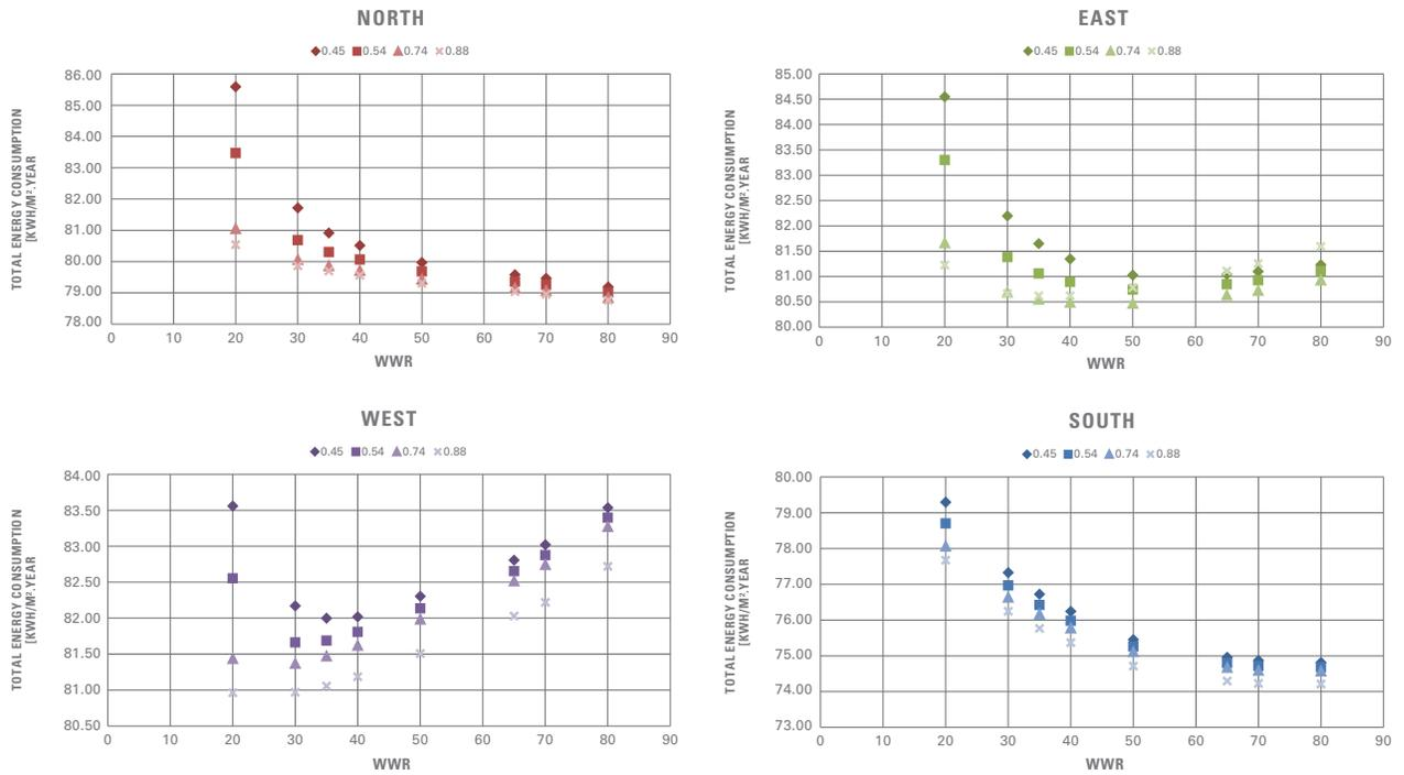
**FIGURE 28** Simulation results for total energy consumption as a function of window-to-wall ratio for different glass transmittance values in Sacramento, California.
