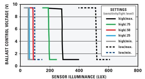
**FIGURE 77** Examples of constant set point algorithms at different sensitivity and light level combinations.
