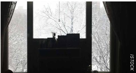
**FIGURE 5** Interior surfaces seen against fenestration may appear as silhouettes due to high contrast between their low brightness and the very bright outdoor surfaces.
