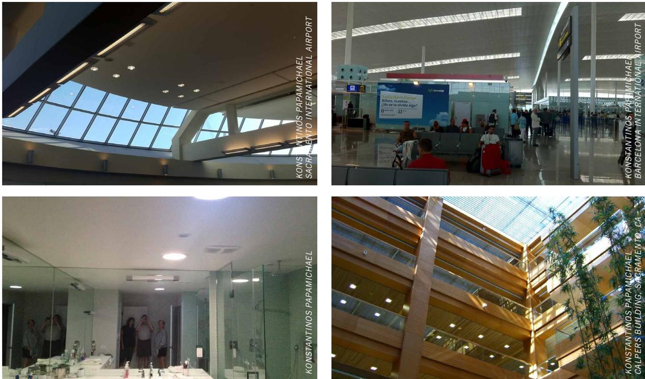
**FIGURE 26** Photographs of different daylighting systems, showing clerestory and vertical windows (top left), skylights and clerestory windows (top right), tubular daylighting devices bringing sunlight through the ceiling (bottom left) and an atrium providing daylight to the space below and the adjacent spaces on each floor (bottom right).
