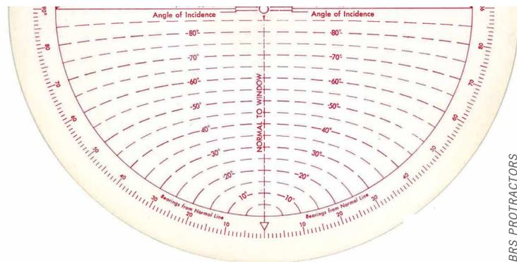
**FIGURE 35** Incident angle iso-contours for a vertical surface. Usually used as overlay on sun path diagrams to quickly estimate solar incident angles on vertical surfaces.
