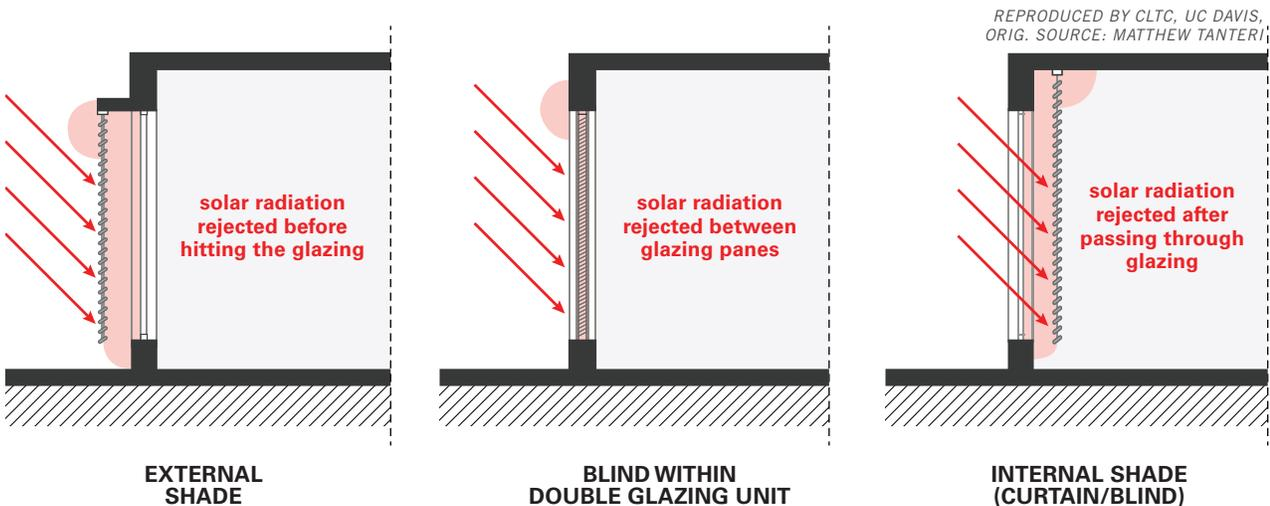
FIGURE 51 Schematic drawing showing the effect of a shading device placed on the exterior of the glazing system (left), between glazing panes (center) and on the interior of the glazing system (right).
