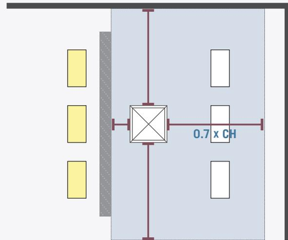
FIGURE 66 Example electric lighting and daylighting design used to show how to calculate a skylit zone with varying obstruction heights.
