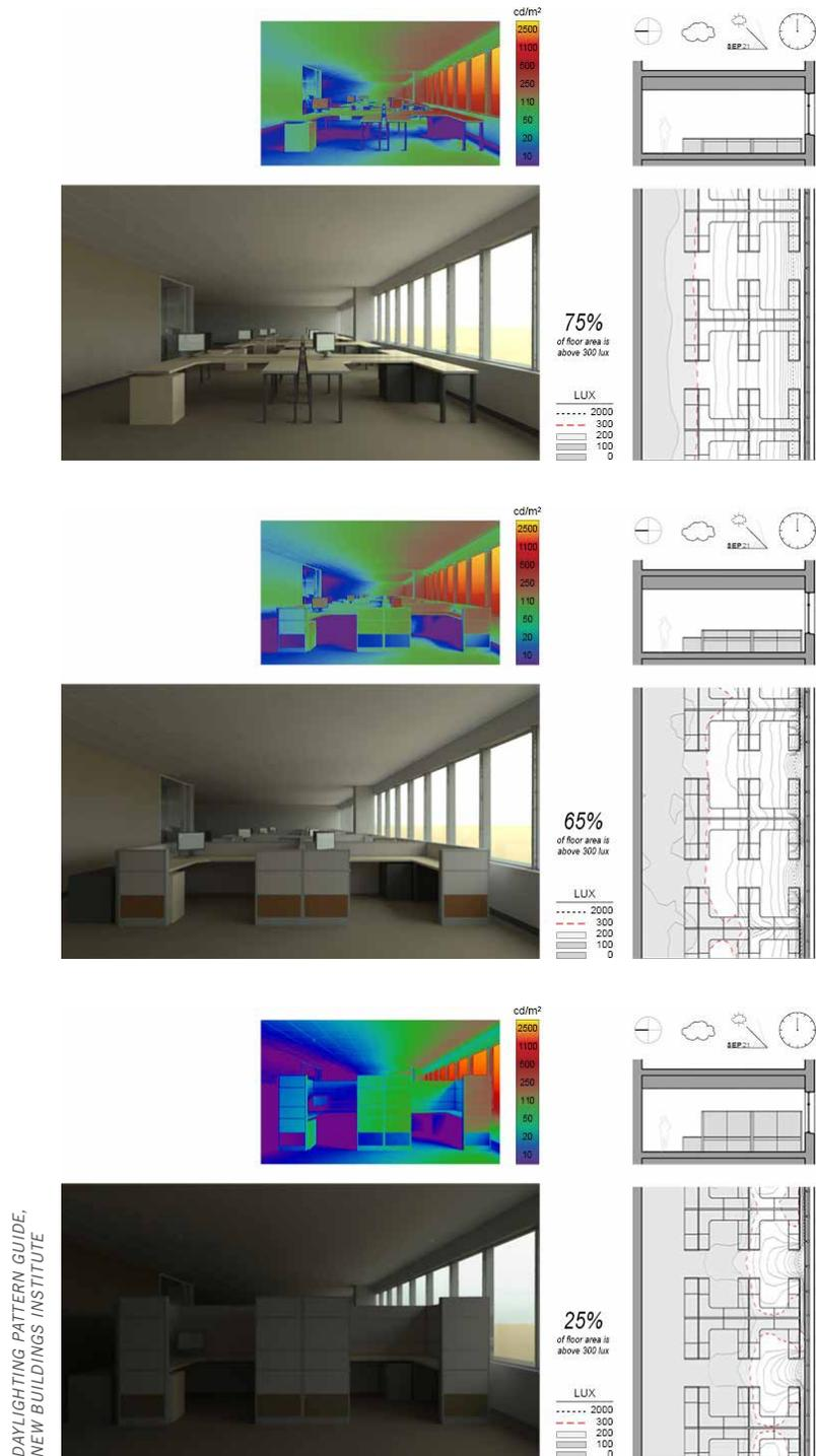
FIGURE 62 Series of computer-simulated renderings showing the effect of furniture on daylight performance under overcast skies.
