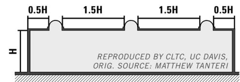
FIGURE 31 Schematic drawing showing rule-of-thumb spacing for skylight applications.
