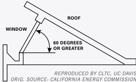
**FIGURE 21** Schematic drawing showing the Energy Code definition for windows.
