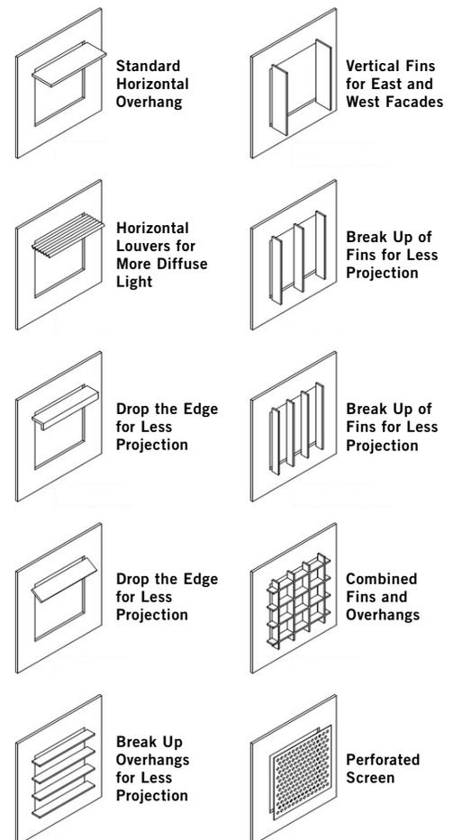
**FIGURE 53** Schematic drawings of horizontal and vertical exterior shading devices.
