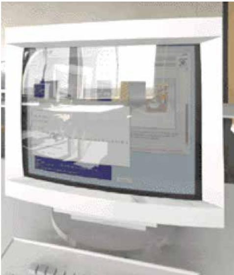
**FIGURE 4** Glare from veiling reflections off a computer monitor, that compete with the brightness of the screen, producing visual discomfort.
