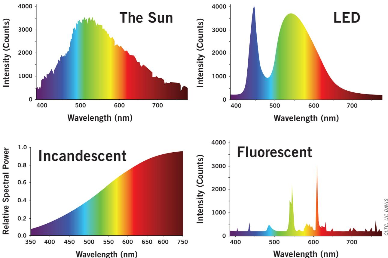
FIGURE 1 Spectral power distribution refers to "the radiant power emitted by a light source over a range of specified wavelength," typically the visible range (approximately 360 to 830 nm).
