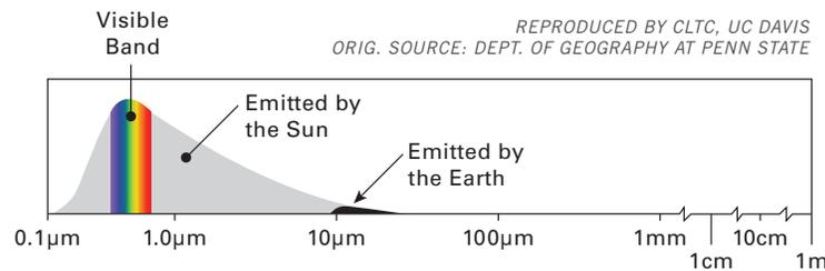
**FIGURE 8 LEFT:** The spectral power distribution of solar radiation and the distinction between near and far IR radiation. The lower the temperature of an object, the longer the wavelength of the IR radiation it emits. The wavelengths of radiation emitted by the earth are more than an order of magnitude larger than the wavelengths emitted by the sun.
