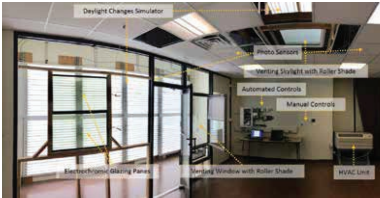
Figure 1. CLTC's Integrated Building Controls Laboratory (IBCL), shown without wall elements on the façade to allow view of the daylight-changes simulator.
