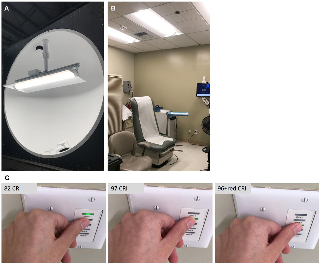
Fig. 1. Example of the (A) LED luminaire used, (B) installed in the ceiling of an exam room at a single, tertiary, academic dermatologic practice, and (C) photographs of normal skin under lighting provided by the three LED sources studied.
