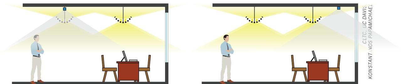
**FIGURE 73** Schematic drawings showing ineffective placement of photosensors that result in unreliable sensing of daylight changes (left) and electric lighting changes (right).
