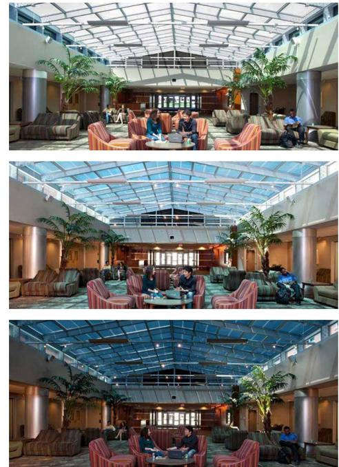
FIGURE 47 Photographs of atrium with electrochromic glazing at high (top), medium (middle) and low (bottom) transmittance states.
