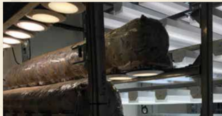
Figure 1. Test rack showing downlights with LED A-lamps (left) and 4-ft indoor fixtures for linear LED lamps (right)
