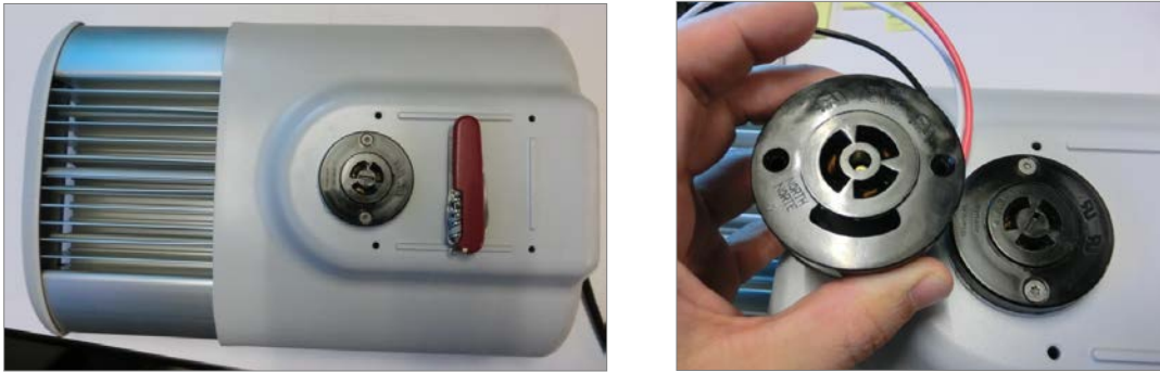
Figure 17: Original ANSI 136.10-2006 Receptacle (left); Manufacturer Specific Receptacle (right)
