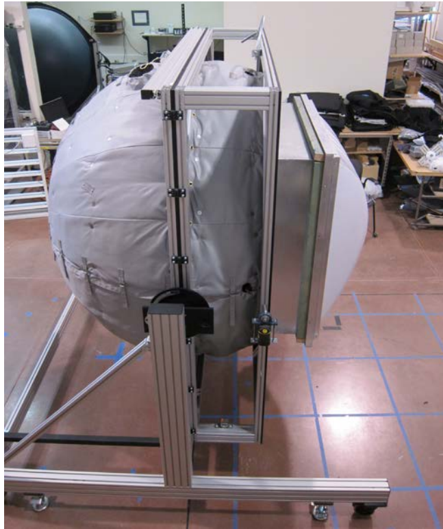
Figure 30: Commercial Skylight with Louvered System Mounted to Custom Integrating Sphere
