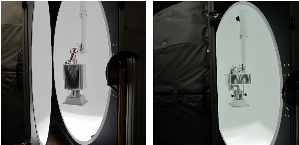
Figure 9: Evaluation of a Plasma High Bay Luminaire at CLTC Test Facility
